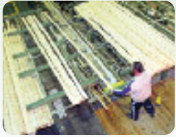
2001: New mill installed at Lingfield featuring a high speed Weing moulder with automated handling.
