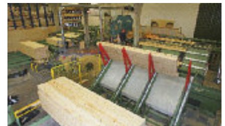
New automated, high speed Stenner re-saw line - Lingfield
