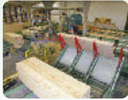
2005: New mill installed at Lingfield featuring a high speed Stenner re-saw with automated handling.
